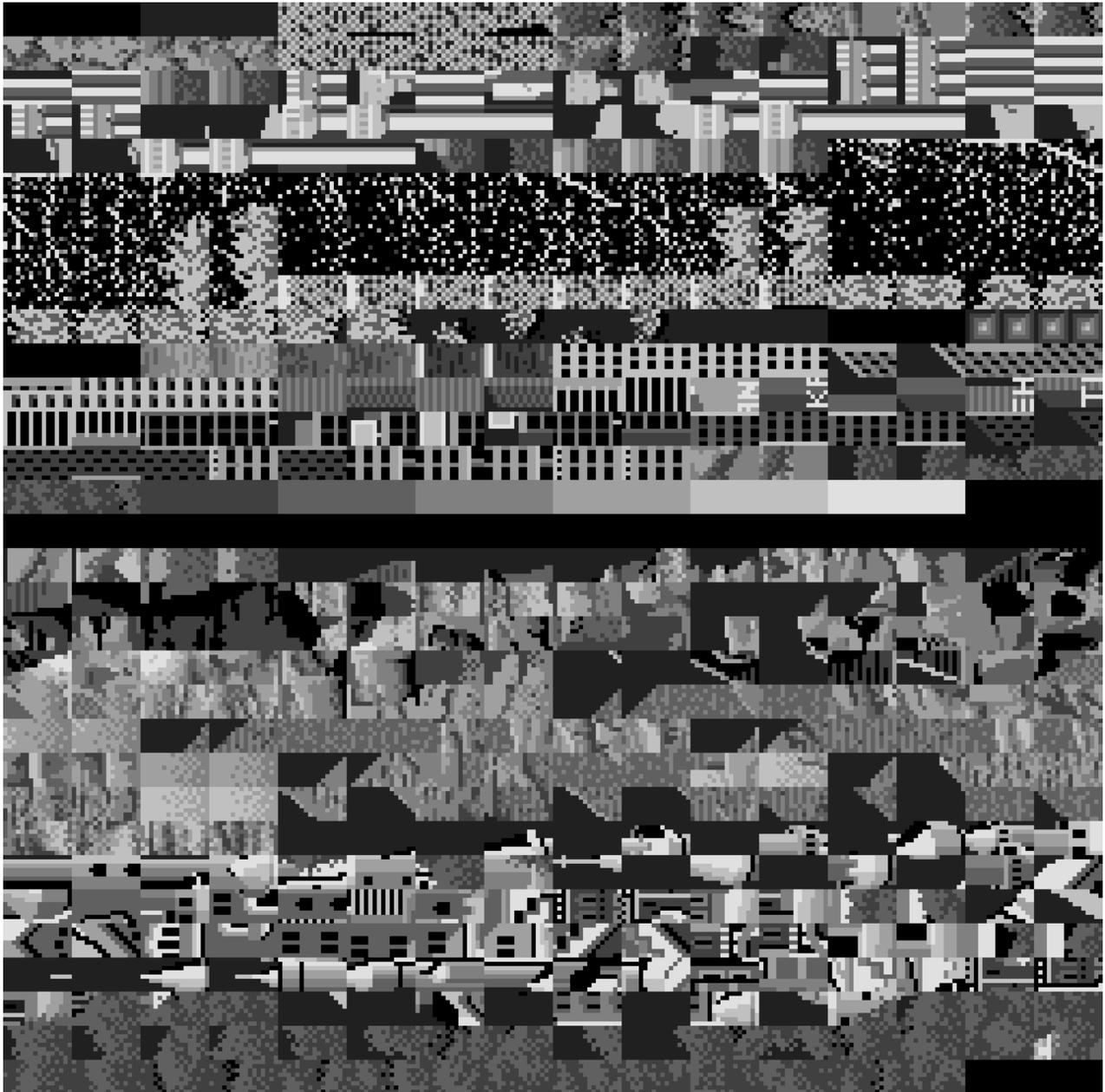
And finally the sprite tile ROM. The 16x16 sprites take up the upper half, and the 32x32 sprites the lower half.
